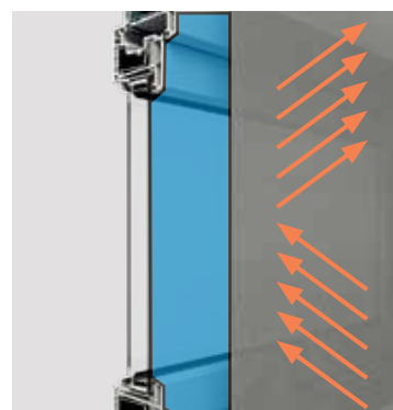
Exterior sun screens are very effective: many fabrics reflect more than 60% of the sun's rays.
